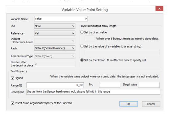
Simply by Clicking OK, the DT10 Software inserts an optimized Test Point into the source code to perform the automatic validation of the data at runtime
