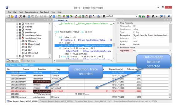
DT10 will also provide you with a Function Trace report, with a graphical illustration of the embedded software behavior, including the relationship and timing between function calls; all to facilitate the diagnosis and correction of the software bug.
